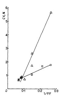
Fig.3. Plot of coefficient of variation of tablet weight versus reciprocal of flow factor. Single punch tablets,  $\Delta$ : multiple punch tablets, .
