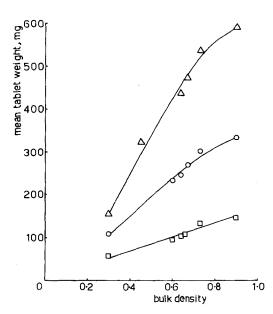
Fig. 1. Plot of mean tablet weight against bulk density for tablets compressed on the single punch machine using 8mm, O, and 10mm,  $\Delta$  , punches and on the multiple punch machine using 5mm punches, \sim .
