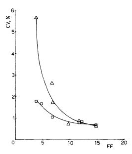
Fig.2 Plot of coefficient of variation of tablet weight versus flow factor. Single punch tablets,  $\Delta$ ; multiple punch tablets, D.
